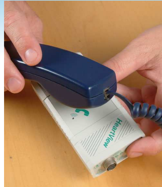
Acoustic transmission of ECG via phone
